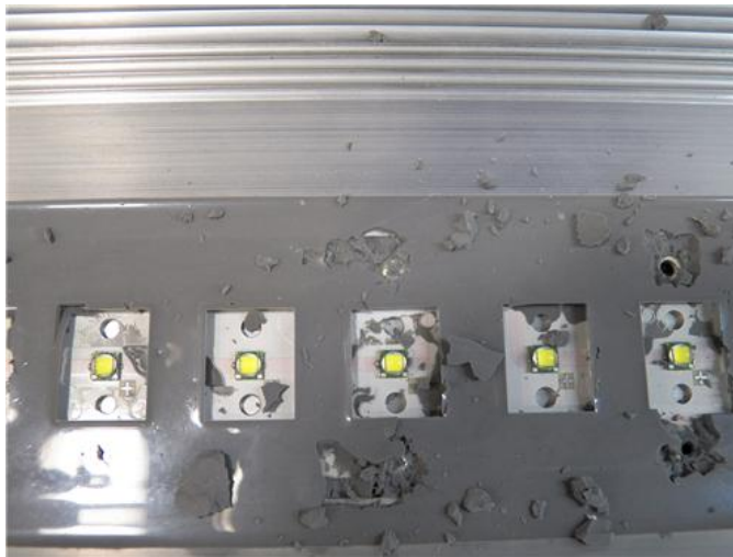
Figure 22: Potting material under lenses
