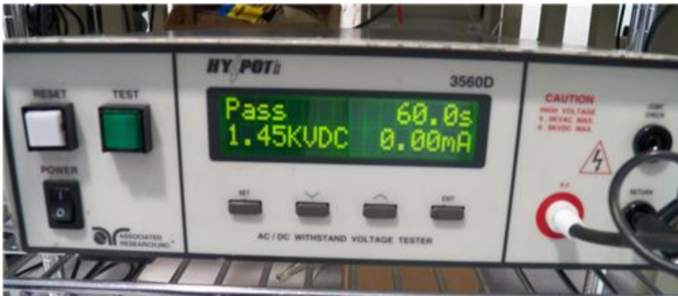
Figure 13: Dielectric Withstand Test Result
