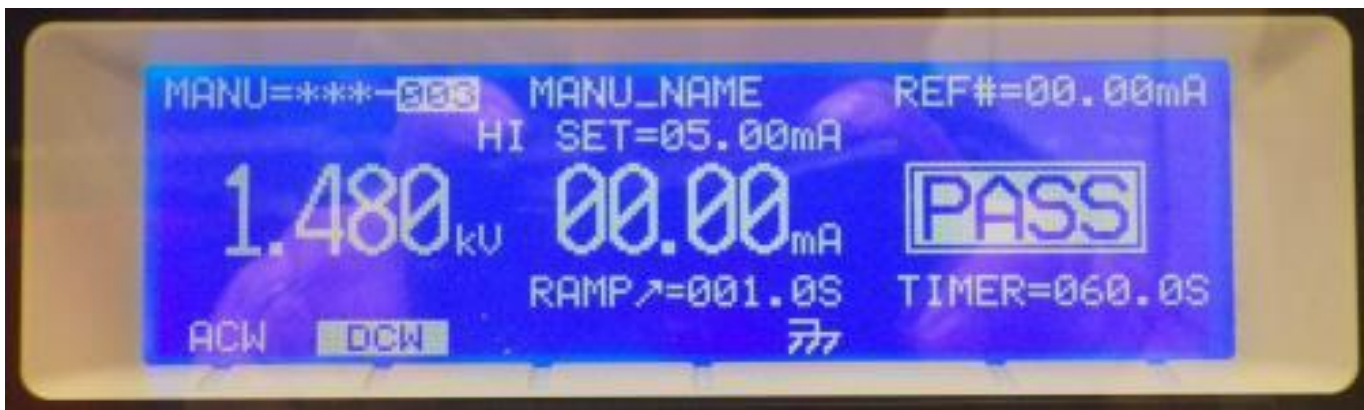
Figure 11: Dielectric Withstand Test Result
