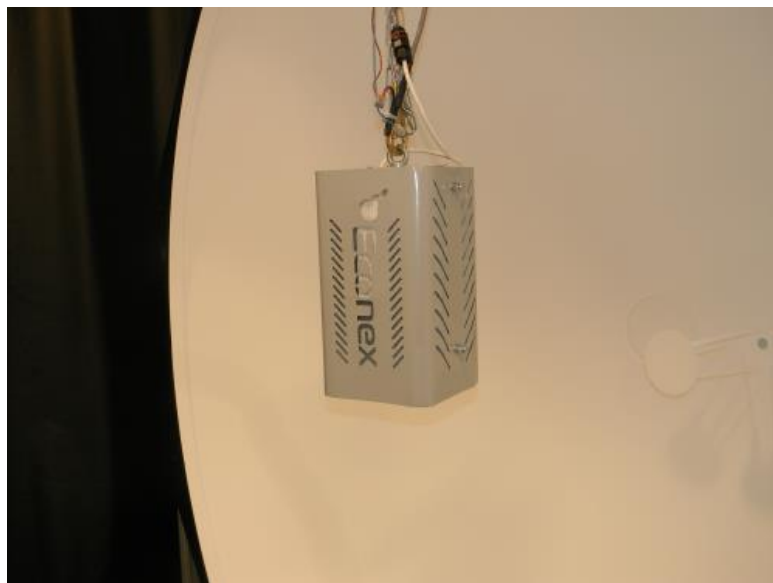
Figure 3: Sample in 2m Integrating Sphere
