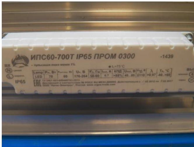
Figure 7: Picture of LED driver
